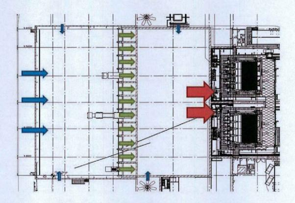
When the doors to the tipping hall are opened to allow lorry movements, air is drawn in via the open doors supplemented, where required, by smaller quantities of air drawn through the louvres at the back of the tipping hall.
